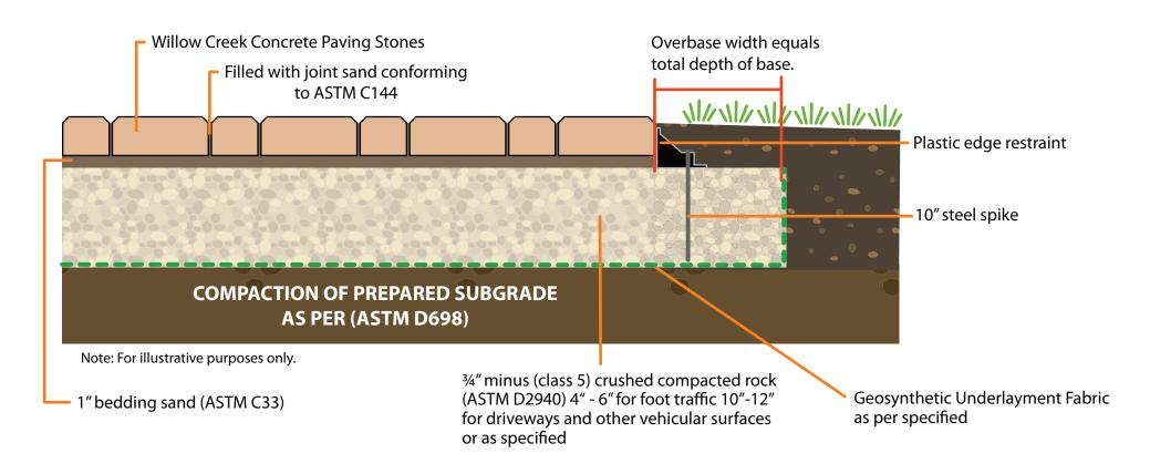
Typical Cross Section of Concrete Pavers on an Aggregate Base for Residential Pedestrian and Vehicular Applications
