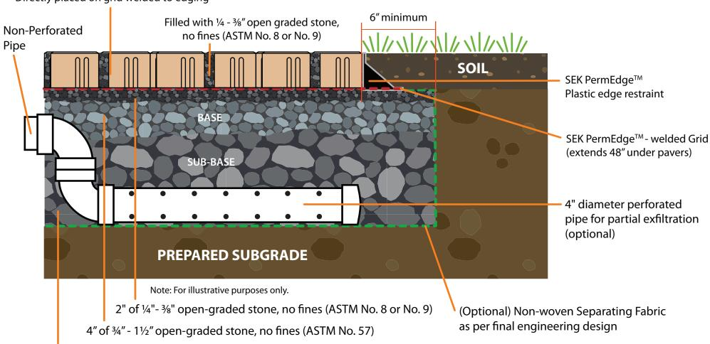
Aqua-Loc<sup>®</sup> Permeable Pavement System Residential Pedestrian and Vehicular Cross Section Using SEK PermEdge™
