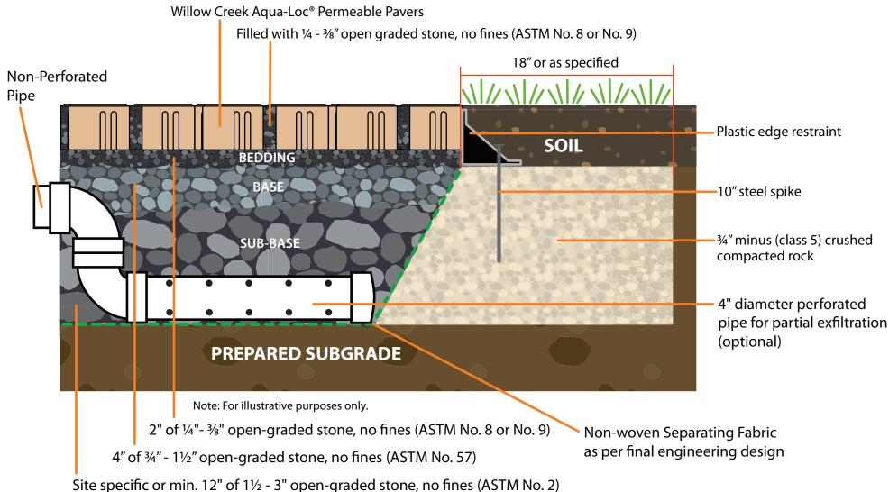
Aqua-Loc® Permeable Pavement System Residential Pedestrian and Vehicular Cross Section
