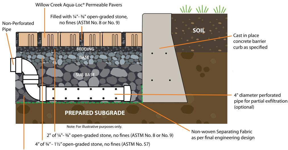
Site specific or min. 12" of 1<sup>1</sup>/<sub>2</sub> - 3" open-graded stone, no fines (ASTM No. 2)
