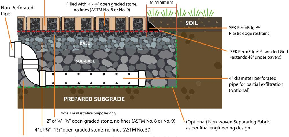
Site specific or min. 12" of  $1\frac{1}{2}$  - 3" open-graded stone, no fines (ASTM No. 2)
