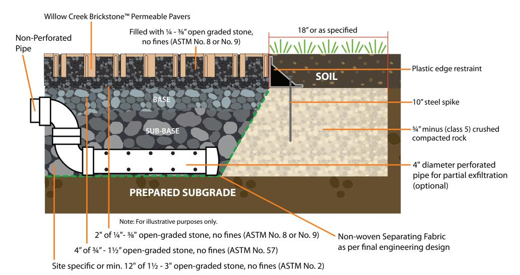
Brickstone™ Permeable Pavement System Residential Pedestrian and Vehicular Cross Section
