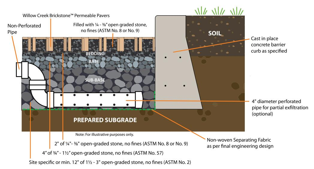
Brickstone™ Permeable Pavement System Vehicular Street and Parking Cross Section
