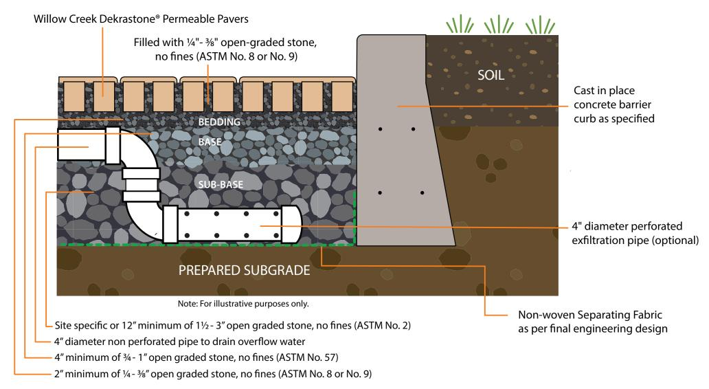
Dekrastone® Permeable Pavement System Vehicular Street and Parking Cross Section
