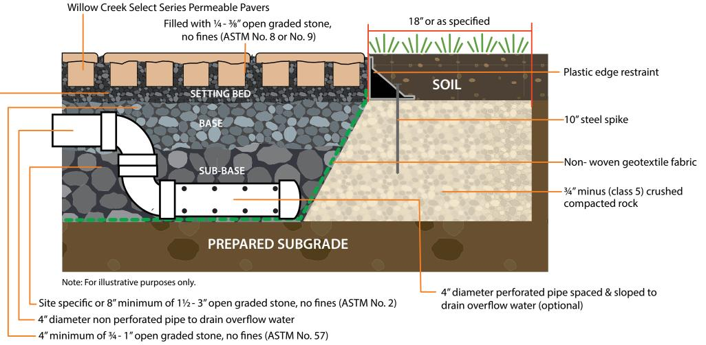
11/2 - 2" minimum of 1/4 - 3/8" open graded stone, no fines (ASTM No. 8 or No. 9)
