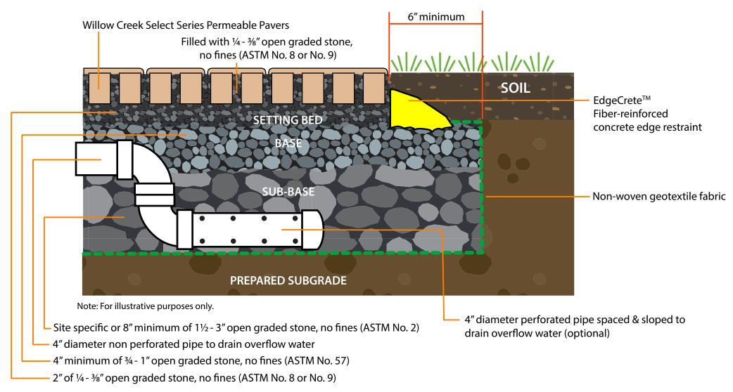
Select Series Permeable Pavement System with EdgeCrete Residential Pedestrian and Vehicular Cross Section
